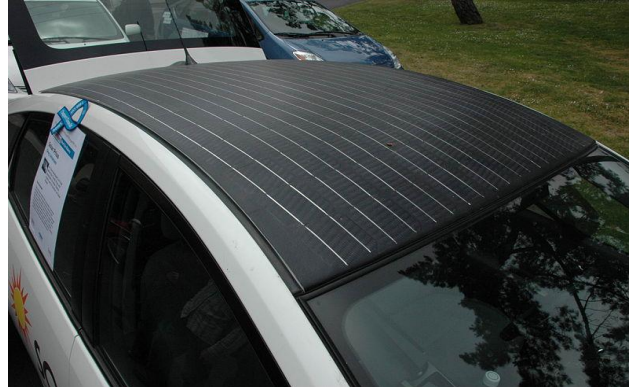
Fig. 6. Photo-cells on the roof of car Prius, 2008
