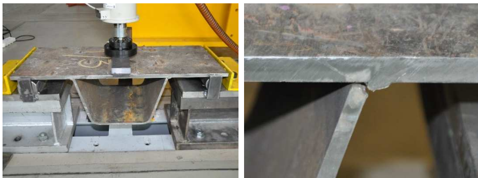
Fig. 4. Detail no.1 under testing: loading scheme (left), typical fatigue failure (right)
