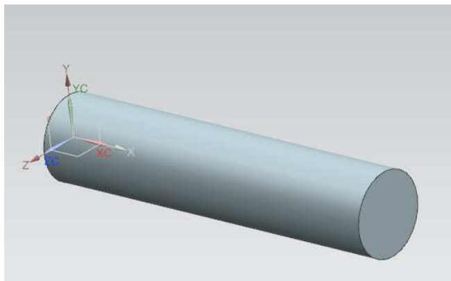
Rys. 3.123. Cylinder – Diameter 45 mm, Height 200 mm
