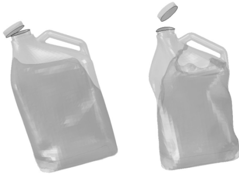
Fig. 2. The water-filled bottle drop-test (CEL model)
