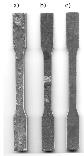
Fig. 2. Tensile specimens – with longitudinal weld (a), transverse weld (b) and base material (c)
