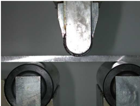
Fig. 3. Scheme of the three rolls bending test
