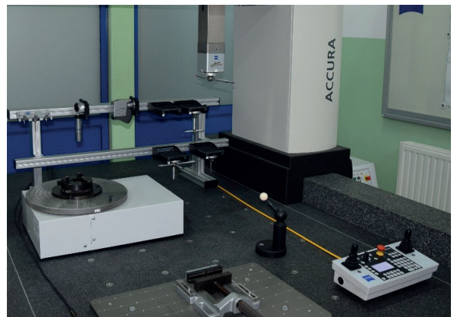
Fig. I.52. Coordinate measuring machine ACCURA II equipped with three measuring probe and a rotary table
