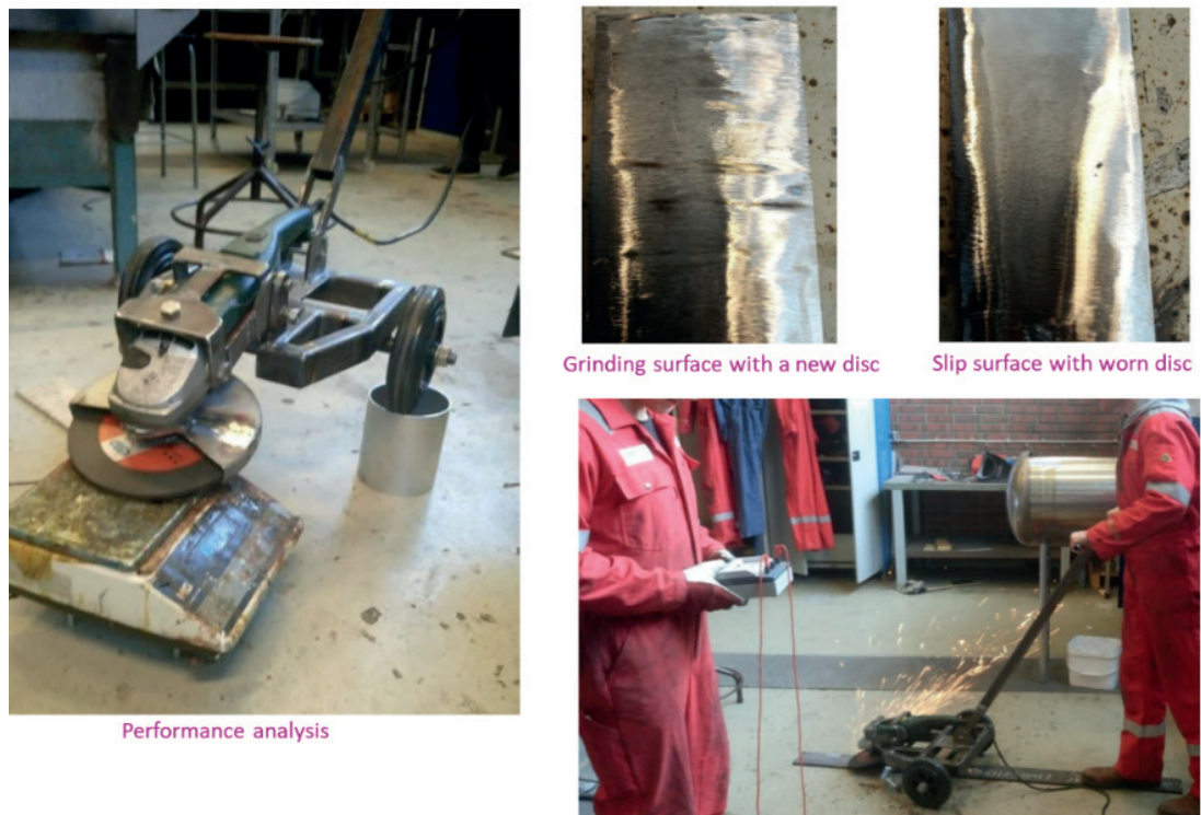
Fig. 2.10. Example of product performance testing
