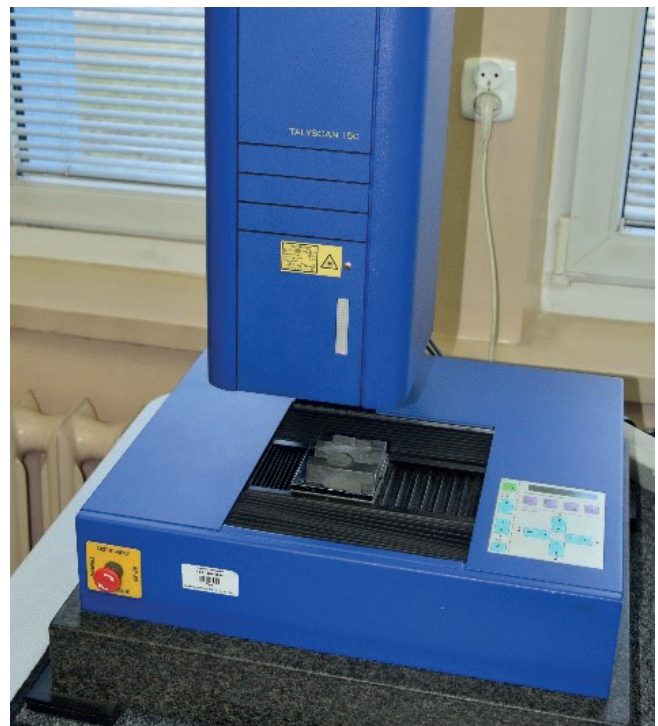
Fig. 1.50. TalyScan 150 dedicated to measurements of roughness
