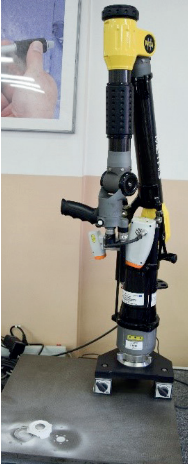
Fig. 1.48. Articulated measuring arm enabling contact and non-contact coordinate measurements and the reverse engineering process
