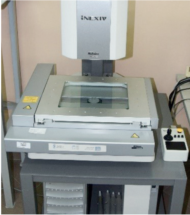
Fig. I.44. iNEXIV measuring system mainly dedicated to 2D non-contact measurements
