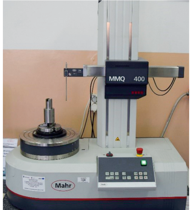
Fig. 1.49. Form measuring system MMQ 400 of the Mahr company applied for measurements of geometrical deviations of products
