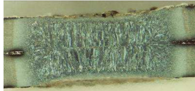
Fig. 3 Macrostructure of sample C (DP 800)
