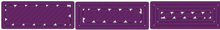
Fig. 4. Tensile test specimens default path generation strategy with one (left), two (middle) and three (right) outlines
