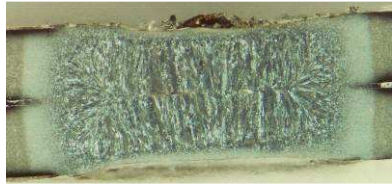
Fig. 1 Macrostructure of sample A (DP 600)
