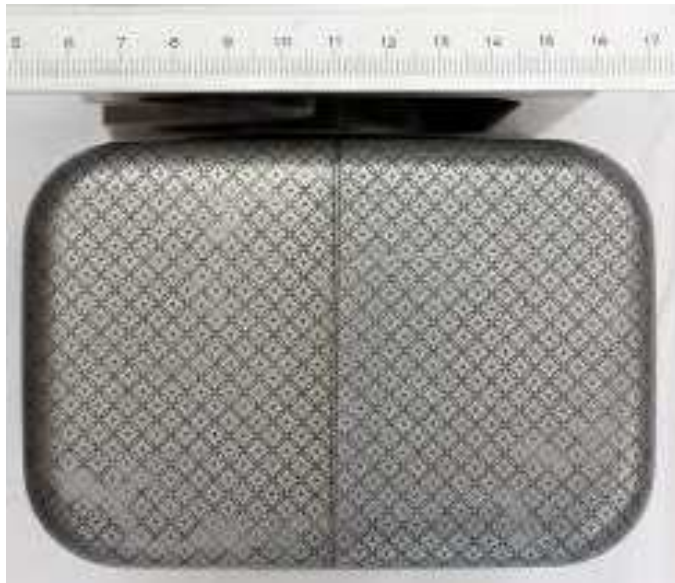
Fig. 3. Bottom of the rectangular box with crosswise oriented weld line
