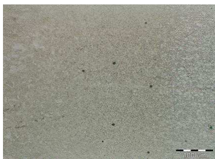
Fig. 9. Microstructure of HAZ of sample F
