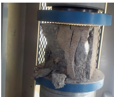
Fig. 2. Concrete samples after compressive strength testing
