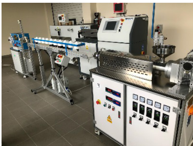
Figure 1. Designed as part of the work author’s line to receive filament.
